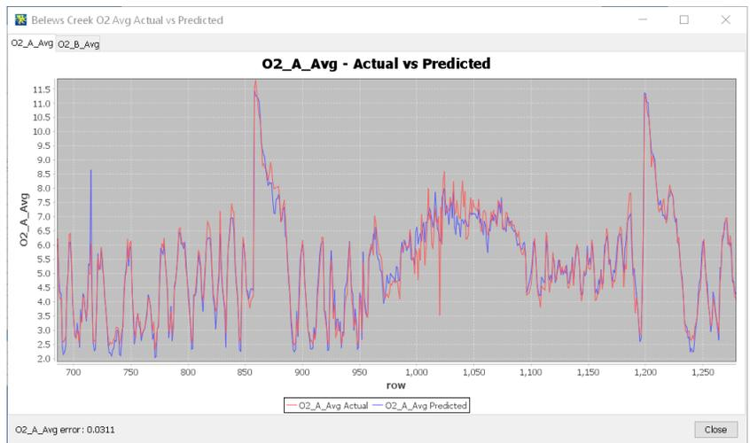
Once the neural network is trained to predict the process value (using user-curated “good” data), it can be used to predict the current value. When significant deviation is observed, users can be alerted to either a malfunctioning sensor, maintenance issue, or some other type of process problem. This method can be applied to any type of output generated by a plant, including entire groups of outputs simultaneously.
